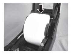
**4.** After pulling out the media, pass the media through the **media guides** and place the leading edge of the media on top of the **platen roller**.
