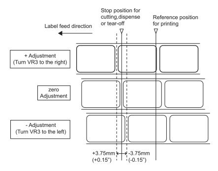
In addition to the above setting, the Offset position can also be adjusted by using SATO Utilities Tool application or by sending command <PO> from the host. The setting range is within ±99 dots.(One exception is for the Tear off mode; for the Tear off mode, the range is -60 dots to +99 dots). This setting is normally not necessary. Use **VR3** potentiometer on the printer for permanent setting.
