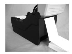
3. While holding the media guide slide lever, adjust the width of the media holder 1 to match the media size. After pulling out the media, pass the media through the media guides and place the leading edge of the media on top of the platen roller.
