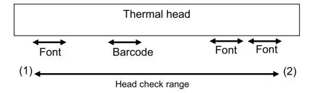
\* The head check will be performed within the minimum and maximum horizontal print area (between (1) and (2)) regardless of print contents.
