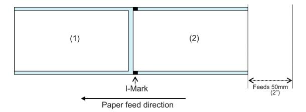
The printer behavior paper end is detected is as follows:
