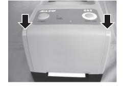
6. After loading the media, turn on the power. The printer is online and the ON LINE (POWER) indicator lights green. When the printer is ready, press the FEED/LINE button to output the leading part of the media.
