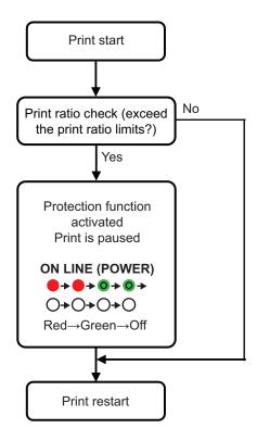
The protection function (pause function) will be activated when the print ratio exceeds the ratio listed in the table below.
