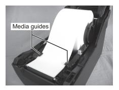
Printed side should face upwards
