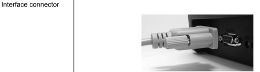
DB-9S or equivalent (Male) Cable length: 5m or less
