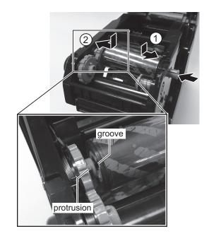
4. In Mount the empty ribbon core on the ribbon wind-up unit the same manner as in step 3 above. When loading the carbon ribbon for the first time, use the empty ribbon core supplied with the printer. However, the subsequent ribbon core can be obtained from the last used up ribbon roll.
