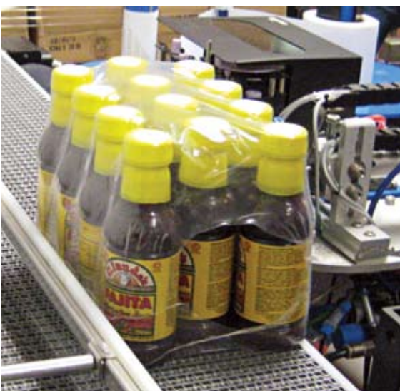
Bundles leaving the wrapper travel past a print-and-apply labeler that applies shipping labels.
