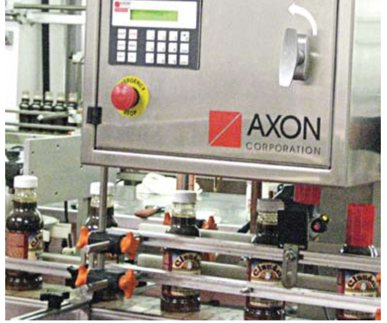
A labeling system applies wraparound UV-coated paper labels to the bottles, left. The labeling system is equipped with two stepper-driven label applicators. The bottles then travel to a tamper-evident bander that applies neck bands that go over the edges of the caps and extend down to the shoulders of the longneck bottles.
