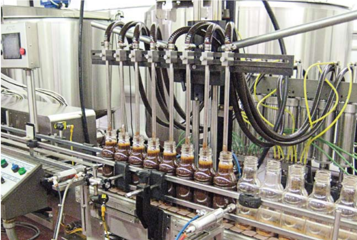
Liquid components are filled on an intermittent-motion, in-line filler that fills eight bottles at a time.
