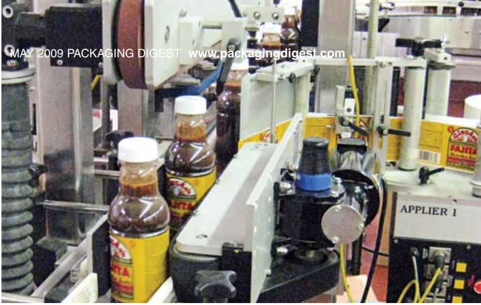
A labeling system applies wraparound UV-coated paper labels to the bottles, left. The labeling system is equipped with two stepper-driven label applicators. The bottles then travel to a tamper-evident bander that applies neck bands that go over the edges of the caps and extend down to the shoulders of the longneck bottles.
