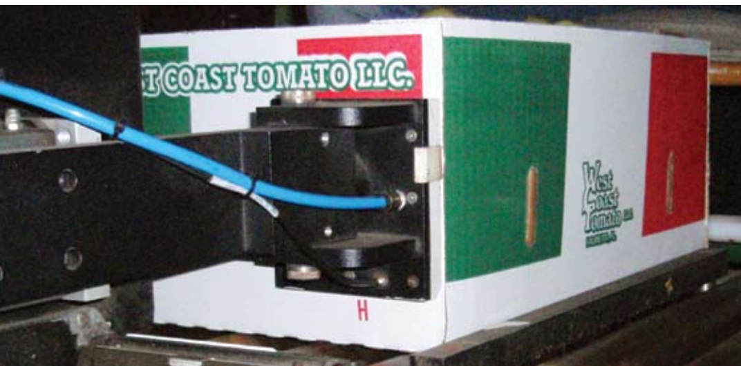
Two different automated fillers, each handling a different type of tomato, feed 25-lb cases of fruit to each line. As those cases merge, photoelectric eyes trigger the print/apply system to produce the correct label, depending on which filler the case came from, and apply it as the case moves down the conveyor.
